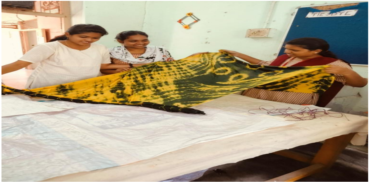
Block printing Tying & Knotting of sari before dyeing
